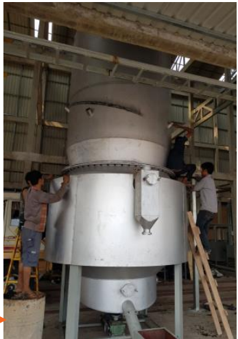
Shell/cake gasifier for electricity and charcoal production →
