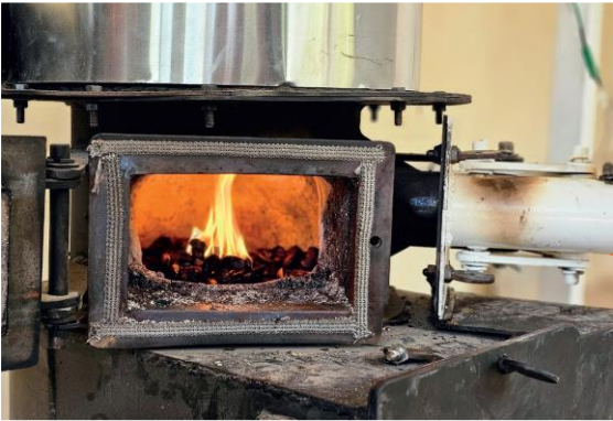
Small shell burner linked to mango drier ↑
