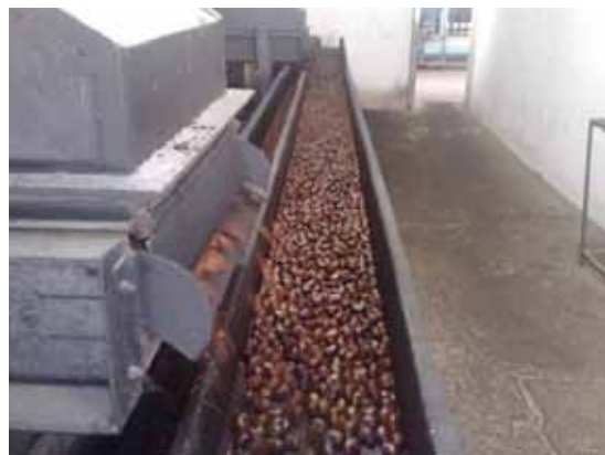
Feeding line after cookers and centrifugal machines
